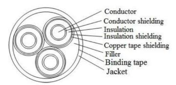
Cable constructure: Conductor: Round Compacted stranded Conductor shielding:semi-conducting XLPE compound Insulation: Cross-Linked Polyethylene (XLPE) Insulation shielding: semi-conducting XLPE compound Copper tape shielding: Copper tape Assembly: For multi-core type cable Binding tape: If necessary Jacket: Lead-Free Polyvinyl Chloride (LF-PVC) Standard: CNS 2655 C2047 Voltage rated: Under 15kV
